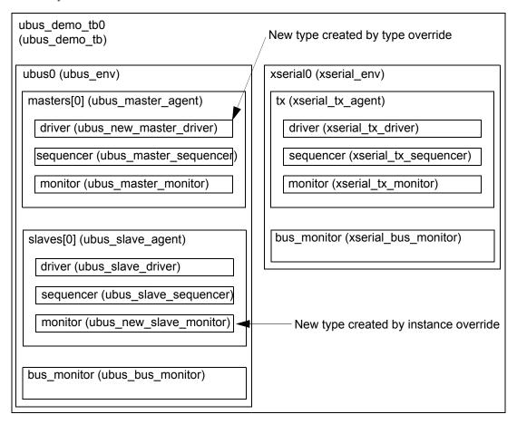
Figure 33—Hierarchy Created with both Overrides Applied
