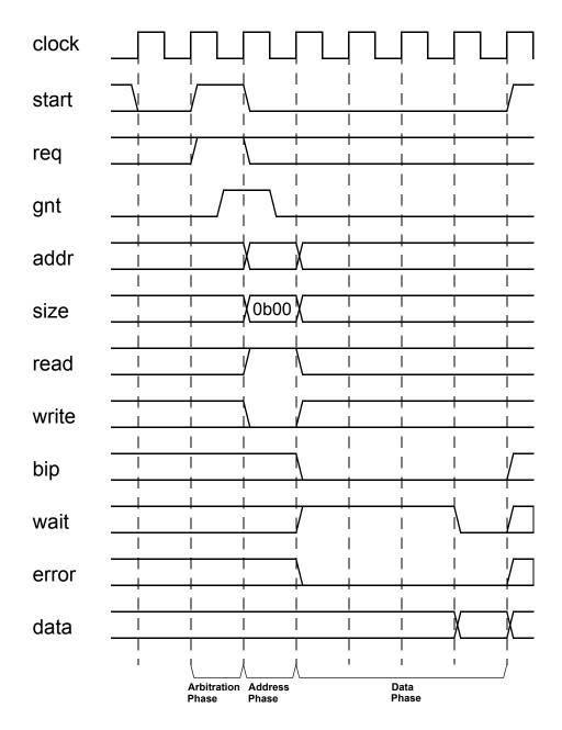
Figure 46—Example Read Waveform
