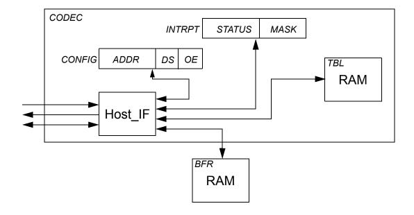
Figure 24—Design Structure of Registers, Fields, and Memories
