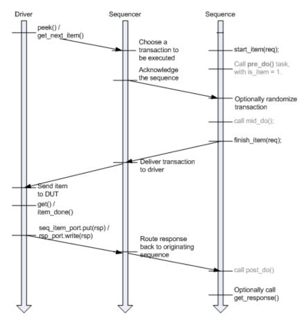
Figure 16—Sequence Item Flow in Pull Mode
