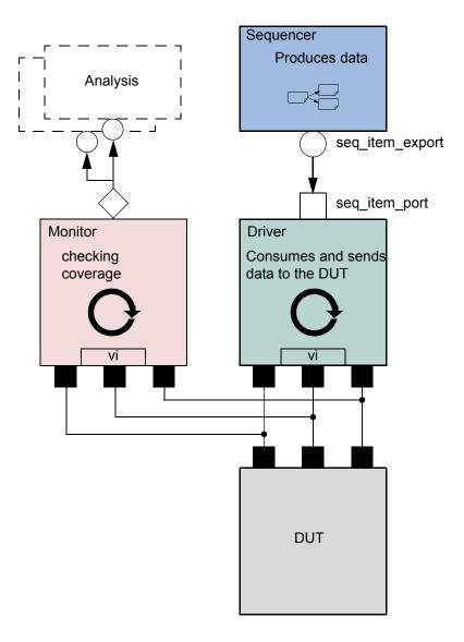
Figure 11—Simplified Transaction-Level Testbench
