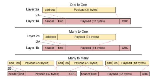
Figure 36—Layer Mapping
