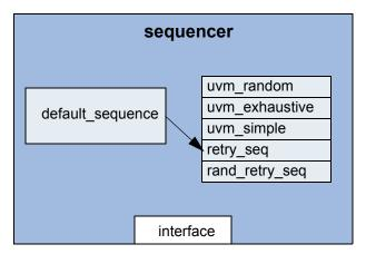
Setting default\_sequence to "retry\_seq" using set\_config\_string("\*.sequencer", "default\_sequence", "retry\_seq"); causes the sequencer to execute the "retry\_seq" sequence
