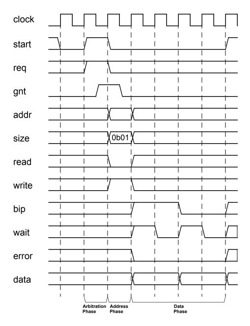
Figure 45—Example Write Waveform
