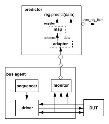
Figure 31—Integration with a Bus Monitor
