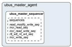
Figure 42—Instance of ubus\_master\_sequencer
