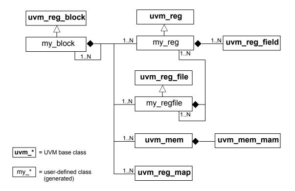
Figure 23—Register Model Class Collaboration
