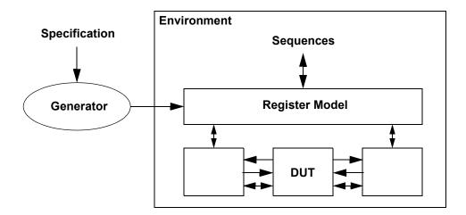
Figure 22—Register Model in an UVM Environment
