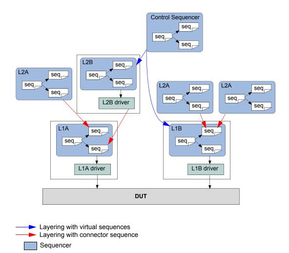
Figure 37—Most-General Case of using Virtual Sequencers
