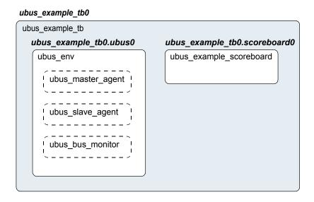
Figure 39—Testbench derived from uvm env
