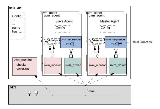
Figure 15—Typical UVM Environment Architecture
