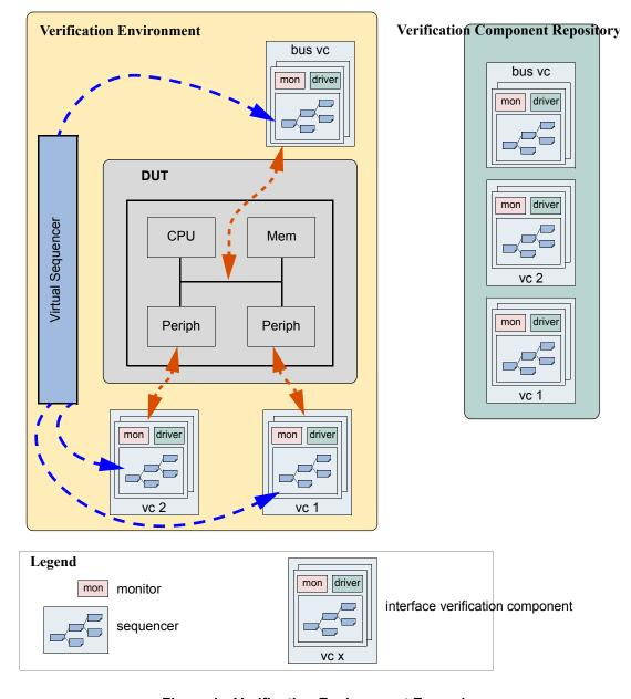
Figure 1—Verification Environment Example
