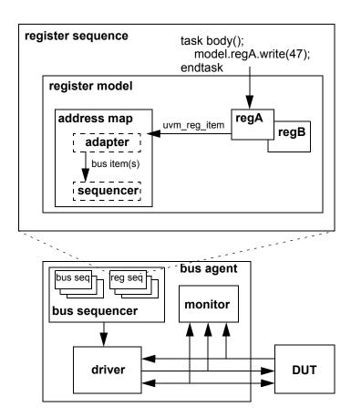
Figure 28—Register Sequence Running Directly on a Bus Sequencer
