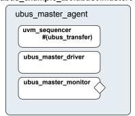
Figure 41—Instance of ubus\_master\_agent
