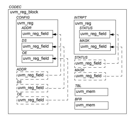
Figure 25—Register Model Structure
