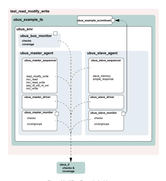
Figure 38—UBus Example Architecture
