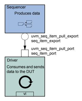
Figure 13—Sequencer-Driver Interaction
