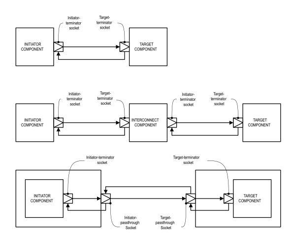
Figure 10—Socket Connections
