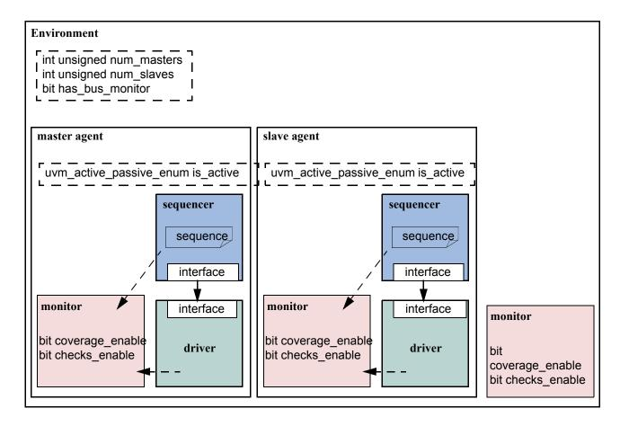
Figure 19—Standard Configuration Fields and Locations
