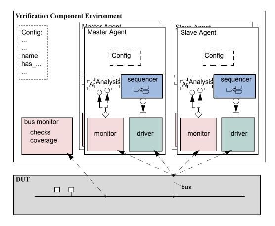
Figure 2—Typical Verification Component Environment
